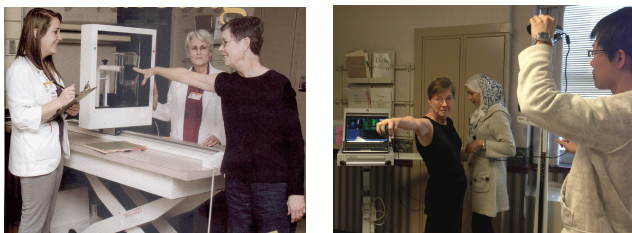
Figure 1. Setup for limb-volume measurement using the Perometry scanner (left) and the proposed IR scanner (right).
